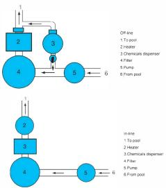
Note: Chemical feeders should always be installed as above indicated position
